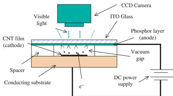
**Fig. 2.** The schematic drawing of the experimental setup used in our lab for measuring the electron field emission properties of the CNT cathodes.
