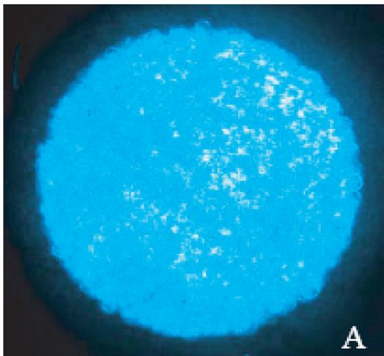
**Fig. 5.** The emission image from one representative 1 cm diameter cathode.
