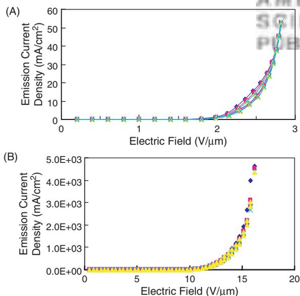
**Fig. 3.** (a) Four consecutive  $J$ - $E$  curves of a FWNT cathode of  $2.5 \text{ mm}$  in diameter measured in DC mode. (b) Four consecutive  $J$ - $E$  curves of a nanotube cathode of  $0.6 \text{ mm}$  in diameter measured in pulsed mode.
