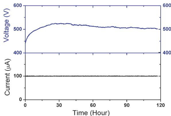
**Fig. 4.** Voltage and emission current versus time curves of a FWNT cathode with  $0.049 \text{ cm}^2$  emission area measured in continuous DC mode.
