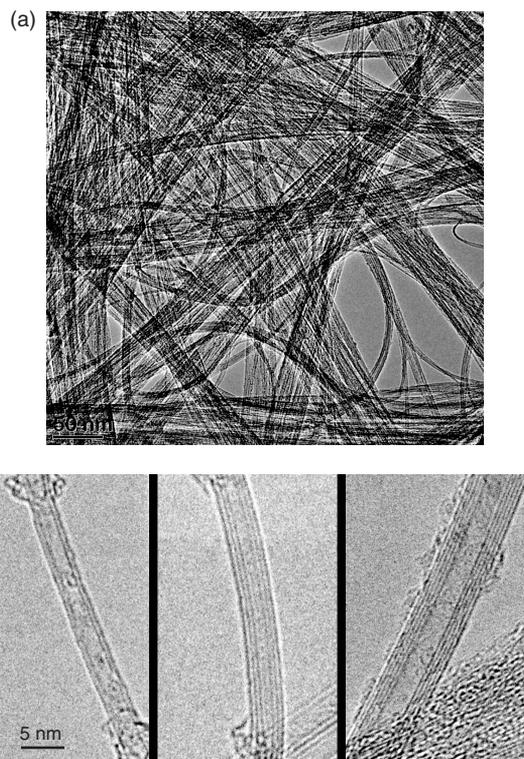
**Fig. 1.** (a) Low resolution TEM image of FWNTs and (b) high resolution TEM images of individual FWNTs with 2, 3, and 5 layers, respectively.
