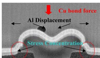
Fig. 8. SEM image illustrating the possible mechanism of aluminum displacement and stress concentration points for a dimple topography.
