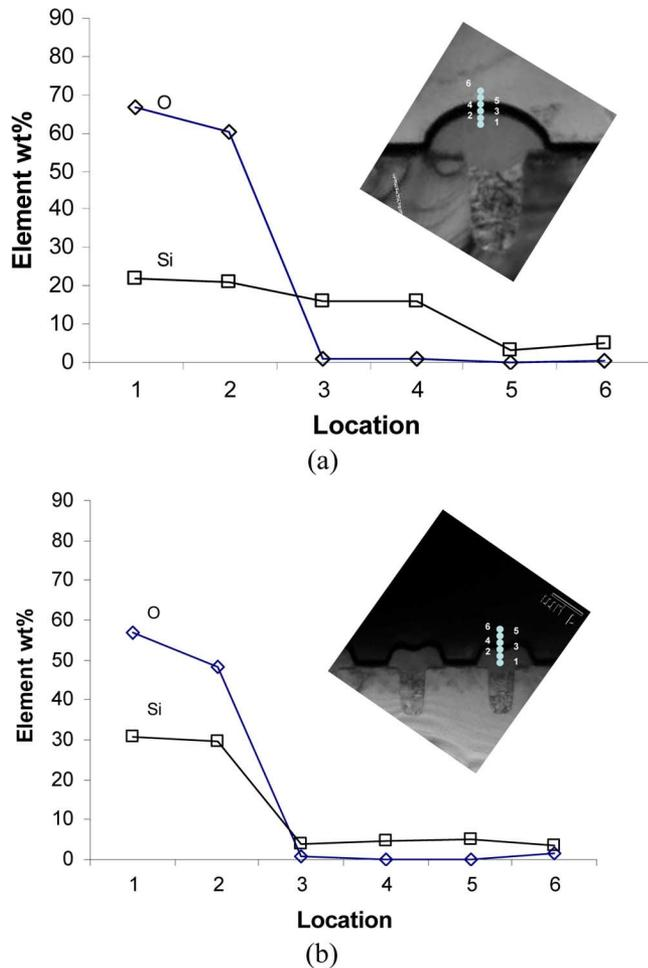
Fig. 10. EDS spectra of oxygen and silicon elemental weight percent at different locations on a cross-sectional TEM sample of (a) round and (b) dimple topography.
