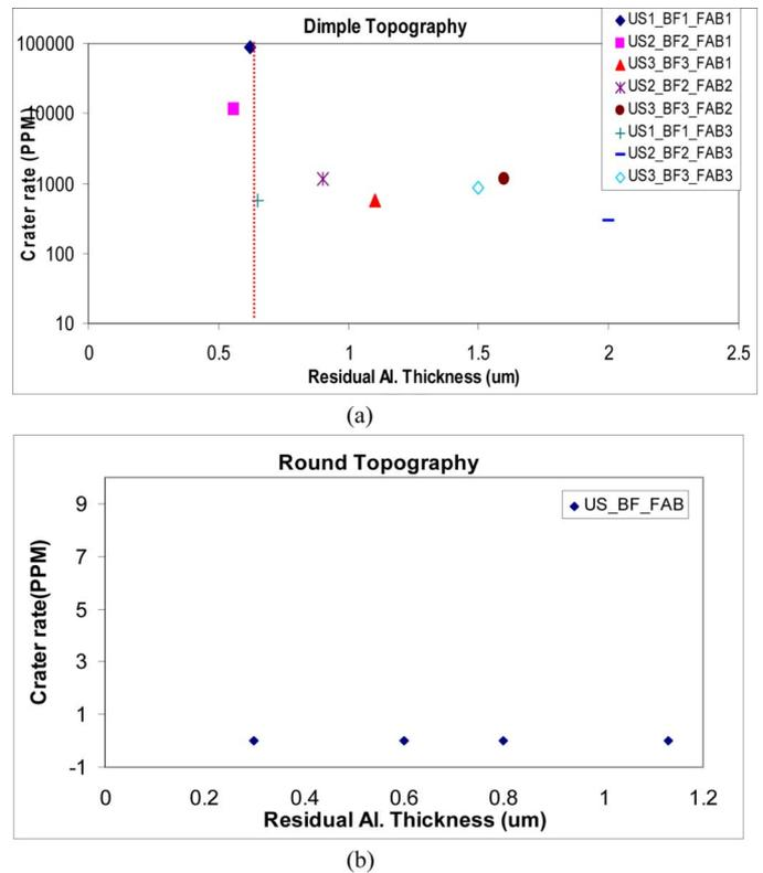
Fig. 11. Cratering rate versus residual aluminum cap thickness for (a) dimple topography with different bond settings and (b) round topography with optimized bond setting.
