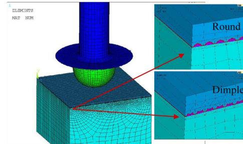
Fig. 1. 3-D FEM mesh showing Cu bonding process for round and dimple topographies.
