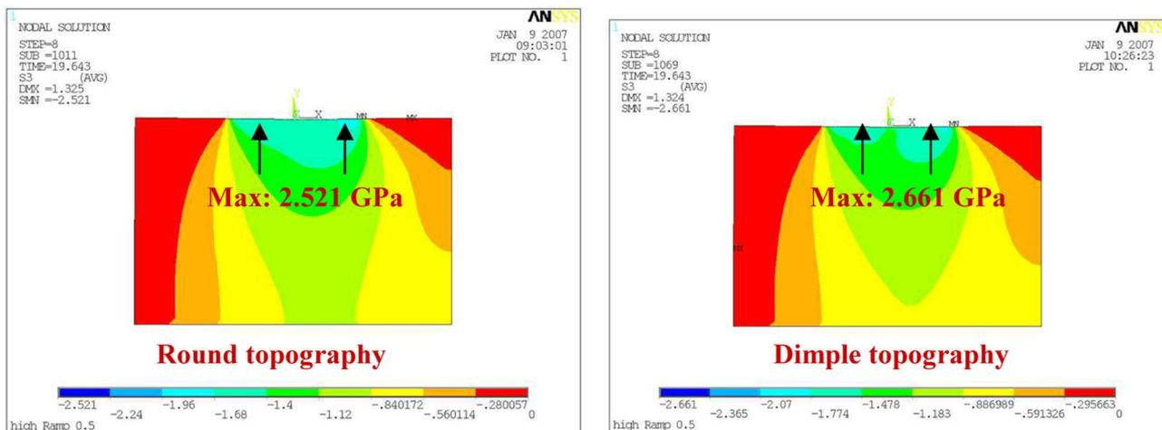
Fig. 6. Stress contours in silicon during Cu bonding process for both round and dimple topographies.
