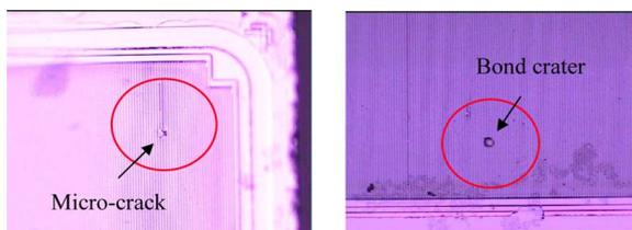
Fig. 7. Micro-cracks and bond craters on silicon observed after etching the top metal and dielectric layers with aqua regia.
