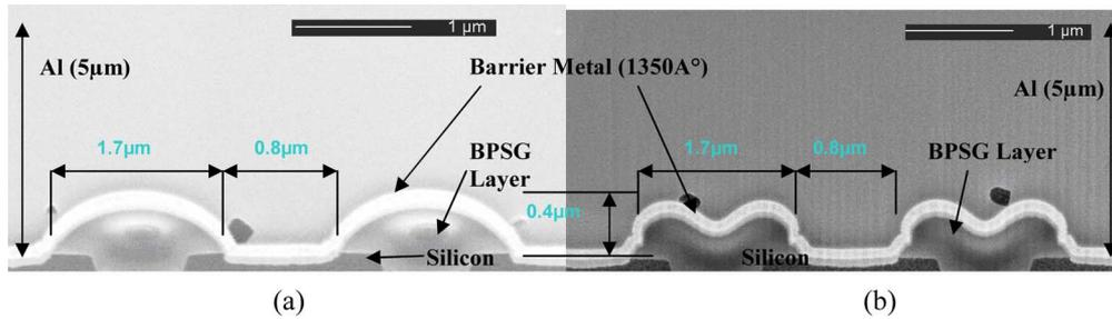
Fig. 2. Cross-sectional SEM images of (a) round and (b) dimple topographies showing aluminum, barrier metal and BPSG layers with their dimensions.
