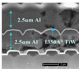
Fig. 9. SEM cross-sectional image of the aluminum/TiW/aluminum sandwich for strengthening the bond pad metal.
