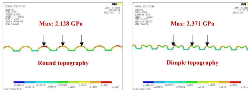
Fig. 5. Stress in barrier/dielectric layers, showing maximum stress concentrations at the top surface region of the barrier metal layer.
