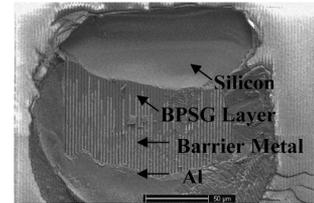
Fig. 3. SEM top-view of a typical silicon crater showing different exposed layers under the aluminum bond pad metal.
