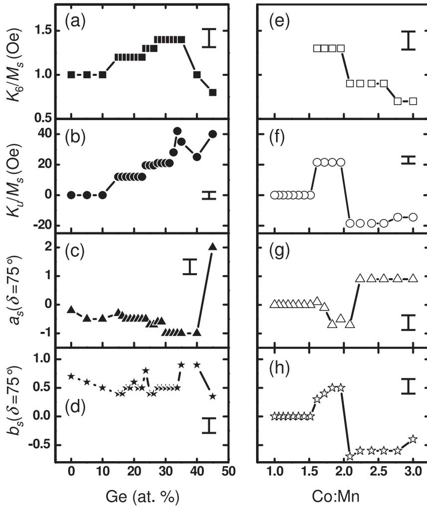
**Figure 9.** Evolution of magnetic anisotropy constants and QMOKE parameters as a function of composition: left column ((a)–(d) from top to bottom), dependence on Ge concentration at a Co to Mn atomic ratio of 2, right column ((e)–(h) from top to bottom), dependence on Co:Mn at 25 at.% Ge. The error bars are shown on the right of each plot.
