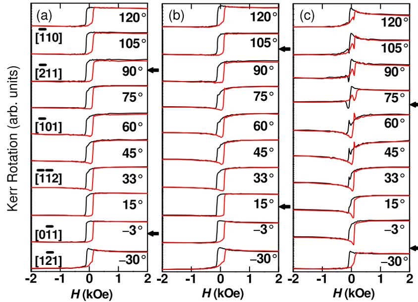
**Figure 6.** Hysteresis loops versus field orientation at various Ge concentrations for  $\text{Co}_x\text{Mn}_y\text{Ge}_z$  at Co:Mn ( $x:y$ ) = 2: (a)  $z = 15$ , (b)  $z = 25$  and (c)  $z = 45$  at.% Ge. Arrows indicate the orientations where hysteresis loops reverse the asymmetry.
