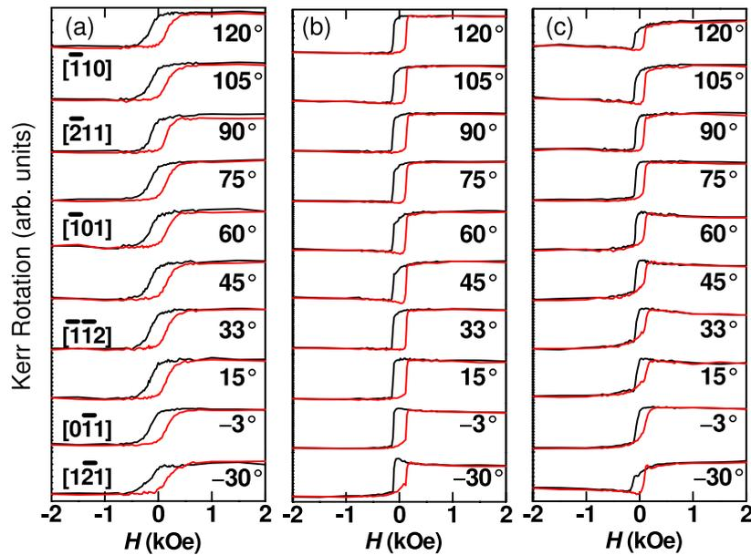
**Figure 7.** Hysteresis loops versus field orientation at several Co to Mn atomic ratios for  $\text{Co}_x\text{Mn}_y\text{Ge}_z$  at  $z = 25$  at.% Ge: (a)  $x:y = 1$ , (b)  $x:y = 2$  and (c)  $x:y = 3$ .
