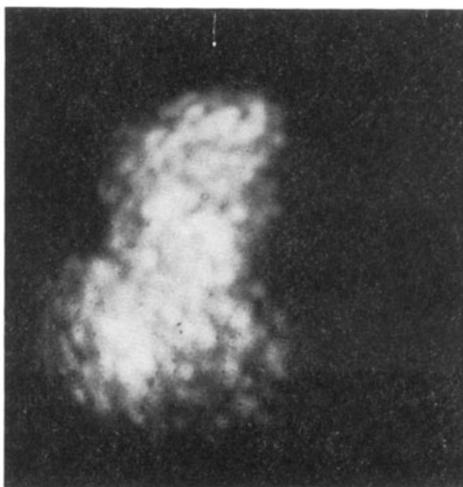
Figure 2. Field emission pattern of tungsten after  $\text{LaB}_6$  had been evaporated on to it (4 kV).
