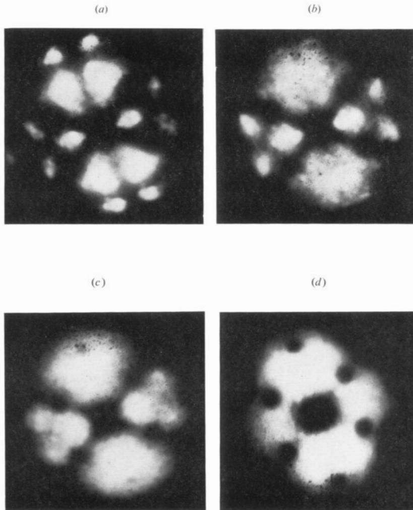
**Figure 3.** Field emission patterns of the same tip at room temperature after it was heated to (a) 1300 °C for 30 s (4 kV); (b) 1900 °C for 20 s (4.2 kV); (c) 1900 °C for 2 min (4.6 kV); (d) after flashing at 2200 °C (5 kV).
