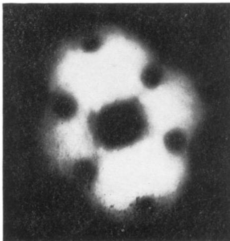
Figure 1. Field emission pattern of clean tungsten (5 kV).
