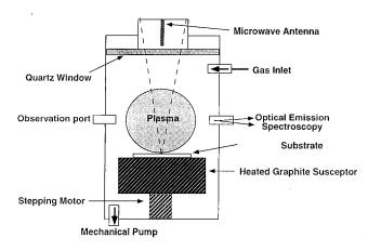
FIG. 1. Schematic of the microwave plasma-enhanced CVD apparatus. Methane and hydrogen gases enter the chamber (with 1 mTorr base pressure) where a coated substrate can be heated to elevated temperature (370-950 °C). The plasma is excited above the substrate on which carbon nanotubes are grown.
