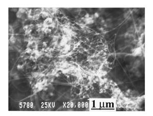
FIG. 2. SEM image of tangled carbon nanotubes of uniform diameter grown on an alumina substrate by microwave plasma-enhanced CVD. Typical diameters of the shown carbon nanotubes are 10-50 nm, while their lengths go well beyond 20  $\mu$ m.
