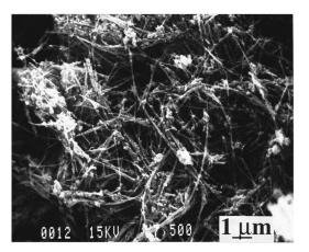
FIG. 3. SEM image of tangled carbon nanotubes produced by the electric arc-discharge technique. Note the striking resemblance in morphology of the arc-produced nanotubes with those produced by microwave plasma-enhanced CVD shown in Fig. 2.
