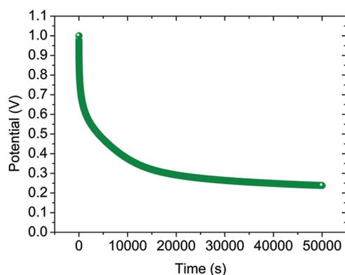
**Figure 7.** Self-discharge of PANI-coated carbon fiber cloth supercapacitor.
