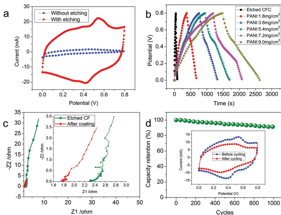
**Figure 3.** (a) CV comparison of same amount of PANI coated on electro-etched and unetched carbon fiber cloth. (b) Charging and discharging curves of electro-etched carbon fiber cloth under various PANI coatings at constant charging current of 2 mA. (c) EIS curve of electro-etched carbon fiber cloth with and without PANI coating. (d) Cycling of PANI coated electrode under constant charging current of 20 mA. Inset is the CV curves before and after cycling.
