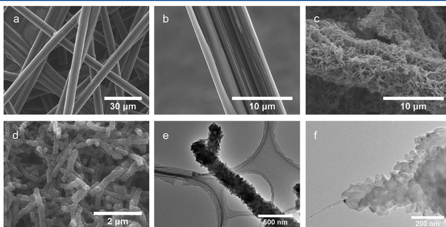
**Figure 2.** (a) SEM image of the carbon fiber cloth. (b) Carbon fiber cloth after electro-etching. Grooves on the carbon fiber are due to electro-etching and the surface area is enlarged. (c) SEM image of electro-etched carbon fiber cloth after PANI coating. (d) SEM image reveals that the PANI coating is composed of tiny nanorods of PANI. (e) TEM image of a PANI nanowire. (f) High-resolution TEM image of PANI nanowire revealing that it is noncrystalline and is porous at the nanoscale.
