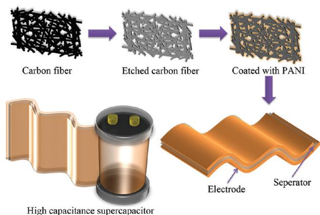
**Figure 1.** Procedure for preparation of carbon electrodes and supercapacitor. Carbon fiber cloth was first etched by electro-etching. The etched carbon fiber cloth was then coated with PANI by electrodeposition. This kind of electrodes can be made into flexible structure that can be rolled into coiled foils.
