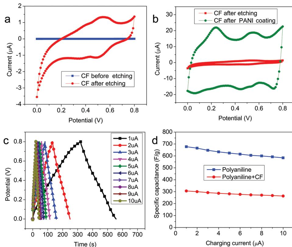
**Figure 6.** Electrochemical properties of a single carbon fiber. (a) CV curves of the carbon fiber before and after electro-etching. (b) CV curves of the single fiber before and after PANI coating. (c) Charging and discharging curves of PANI-coated single carbon fiber under different charging current. (d) Specific capacitance of the PANI coating and the PANI coating together with the carbon fiber under different charging current.
