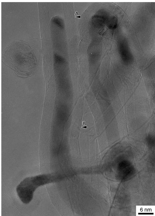
Figure 4 A CVD-grown carbon nanotube encapsulating a filling. The filling was covered completely by a single graphitic shell. There are 11 graphene shells at A and 12 at B.
